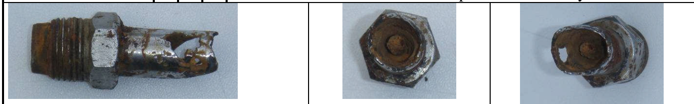
The drinker showing excessive wear Rear of the drinker – partially blocked Front of the drinker with the nipple area rusted off
